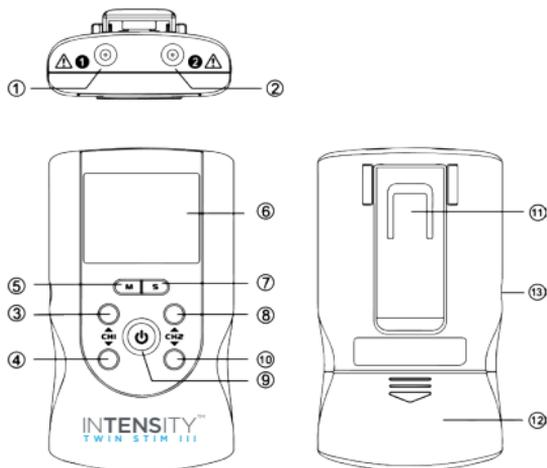
1. Output socket: electric signal output after connection of the cable with adhesive electrodes on channel 1.
